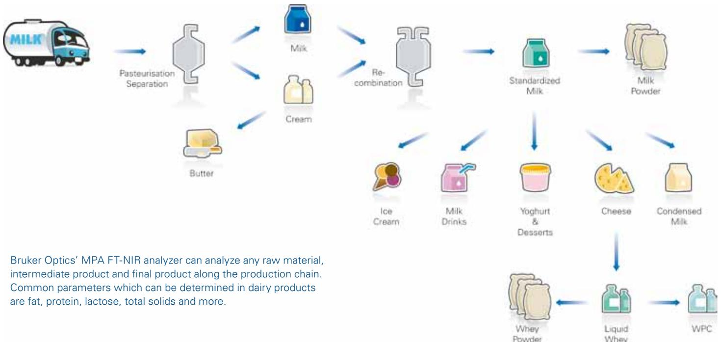
Bruker Optics' MPA FT-NIR analyzer can analyze any raw material, intermediate product and final product along the production chain. Common parameters which can be determined in dairy products are fat, protein, lactose, total solids and more.
