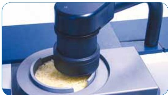
Fig. 4: Measurement of cheese in diffuse transmission.
